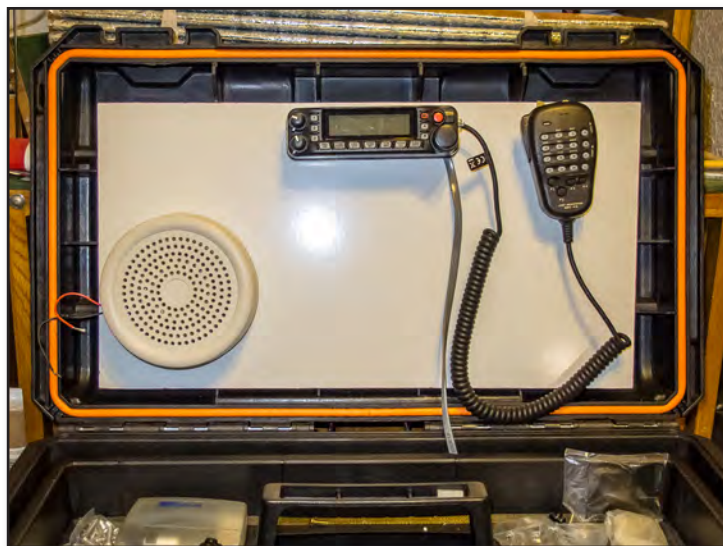
FIGURE 1: The whiteboard with the control head and speaker mounted and installed in the top of the box.
