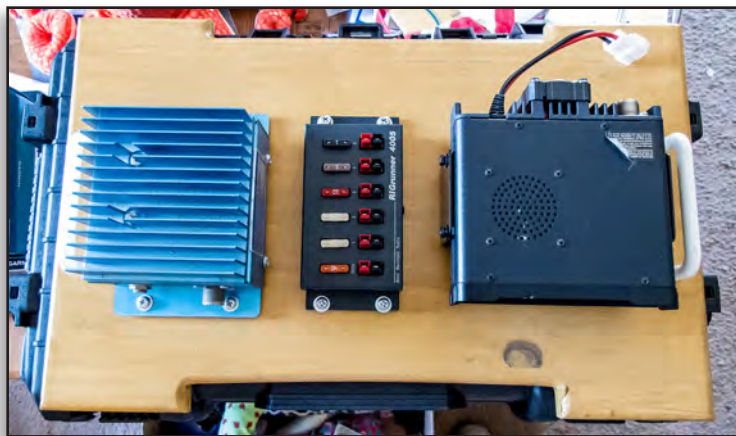
FIGURE 2: The mounting board supports the Henry 2-meter amplifier, RIGrunner 4005 and FT-7900R transceiver.
