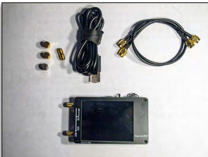
What you get... This is what comes with the Nano VNA. Left to right: Calibration devices, Open, Short and Load. Double ended SMA connector, USB C cable and two connection cables with SMA connectors. Bottom is the Nano VNA itself.
