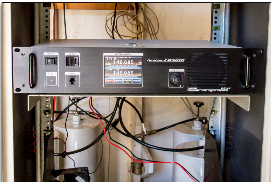
The club's new Yaesu System Fusion® repeater installed and operating at the repeater site. Story and pictures on Page ... John Wright, K6CPO
